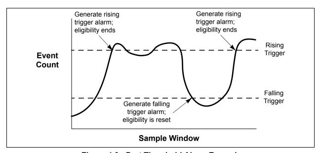
Figure 4-9. Port Threshold Alarm Example
